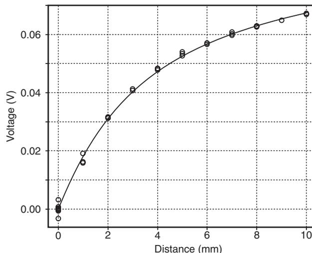
**Fig. 3.** Movement monitor calibration correlating voltage output (V) to distance (mm) between electrodes. Open circles represent voltage recordings at particular known inter-electrode distances, and the line of best fit is described by Eq. (1).
