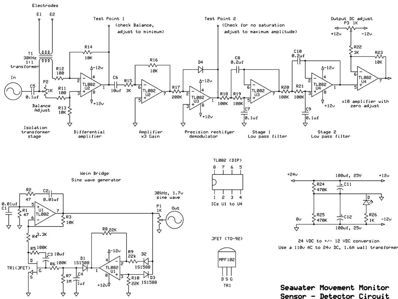
Fig. 2. Movement monitor circuit schematic.
